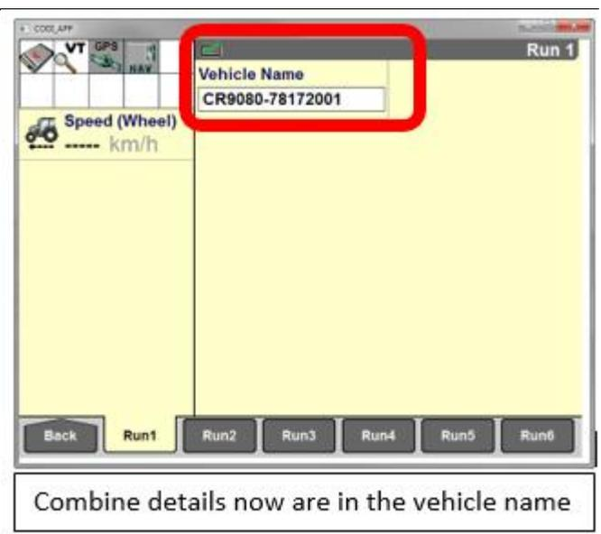
By renaming the monitor name to the model and serial number of your combine it will make it much easier to identify which machine you are using in the software and any generated reports you create
